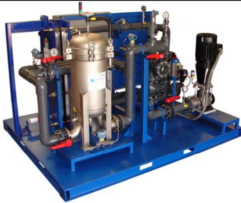
Shown: PCW rated for 300 gpm with 316 SS pump, 304 SS filter housing, 316 SS heat exchanger, schedule 80 PVC. Part # PCW-300-1-1-1-IM-4-PVC.
