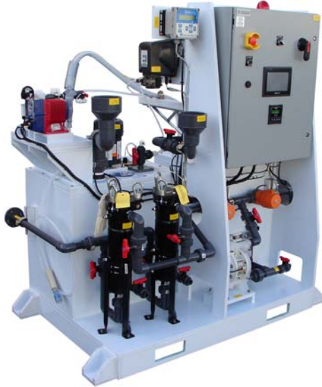
Shown: FRS-NA-10-1-FB-M-IM-1-N4-DL Laboratory 10 gallon single batch tank fluoride removal system without an equalization tank, with day tanks, and a 120 VAC PLC based system.
