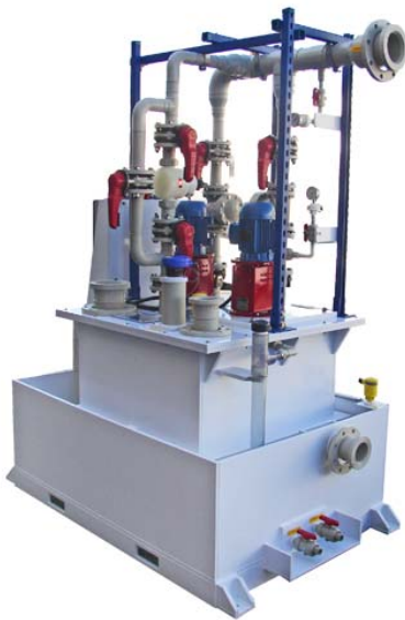
Shown: HCPLS-0300-36-P4-2-AM-4-N4-IC-CL-PP-TC-DC-VM-ST. 200 GPM lift station with 300 gallon tank, duplex pump configuration, polypropylene piping, double containment, and a 460 VAC PLC-based control system.
