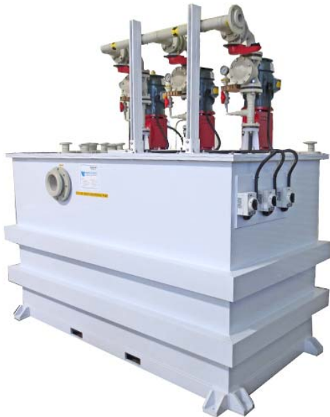
Shown: HCPLS-0700-36-P5-3-AM-4-N4-RC-CL-PP-SC-52-VM-ST. 400 GPM lift station with 700 gallon tank, triplex pump configuration, polypropylene piping, side inlet, and a 460 VAC PLC-based control system.
