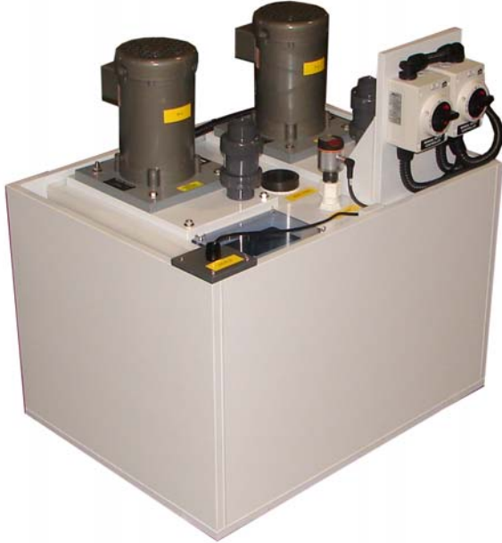
Shown: Duplex 0.5 HP pumps with 32 gallon double contained tank and lockable electrical disconnects for each pump. (DVPLS-32-005-1-P-TC-DC)
