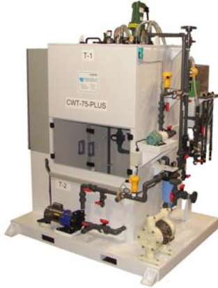
Shown: HMR-150-75-3FP-M-P-1 150 gallon equalization tank, 75 gallon reaction tank, 3 ft 3 filter press, metering pump shelf, 120 VAC PLC based control panel.
