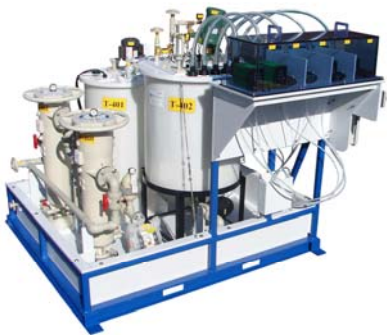
Shown: HMR-100-FB-M-P-1-HX 100 gallon reaction tank with heat exchanger, 2 filter bags, metering pump shelf, 120 VAC PLC based control panel.
