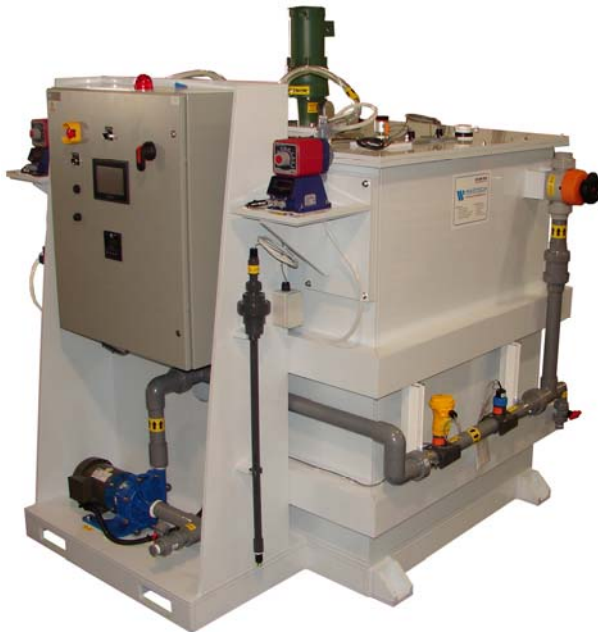
Shown: PDB-500-DC-P-B-IM-4-LR-FL. 500 gallon batch system, acid and caustic addition, discharge flow meter, 460 VAC, IDEC with Maple HMI
