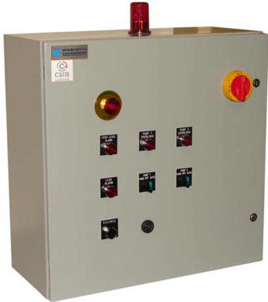
Shown: Duplex 1.5 HP Industrial Pump Control Panel with NEMA 4 enclosure, leak, audible and common alarms. (IPCP-DP-015-4-N4-LA-AA-CA)
