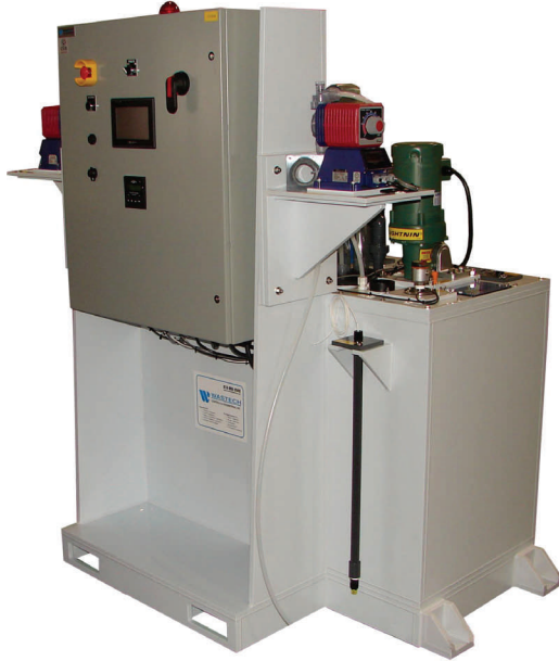
Shown: BATCH-50-SC-B-IM-1-LR. 50 gallon batch system, acid and caustic addition, 115 VAC, IDEC with Maple HMI
