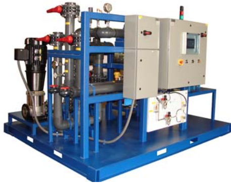
Shown: PCW rated for 500 gpm with 316 SS pump, 304 SS filter housing, 316 SS heat exchanger, schedule 80 PVC. Part # PCW-500-1-0-1-1-PVC
