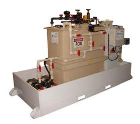
Shown: ADS-H2SO4-100-DC-IM-4-N4-RMP-RDP. 100 Gallon sulfuric acid dilution system with redundant discharge pumps, redundant metering pumps, PVDF dilution tank, 460 VAC control panel, IDEC PLC, and Maple HMI.
