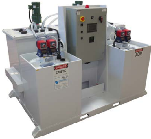
Shown: OMEGA-10-2-SC-G-B-T-IM-1-LR. 10 gpm system, 2 reaction stages, acid and caustic addition, chemical day tanks, 115 VAC IDEC with Maple HMI control panel.
